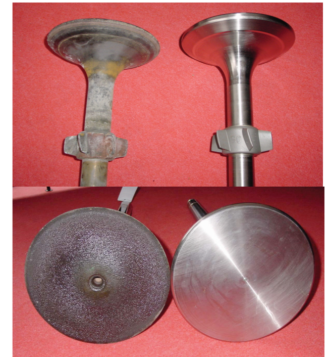
Figure 15 a/b: Nimalike spindle before and after remanufacturing
