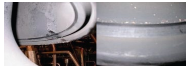
Figure 19: Seat ring and valve spindle show no dent marks after app. 1,000 hours.
