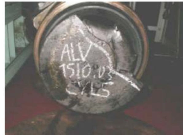
Figure 12: Catastrophic failure of a repaired valve spindle (RTA72 Nimonic-type 740 hrs after repair)
