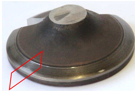
Figure 2: KU Gas engine intake valve after 4,000 operating hours
