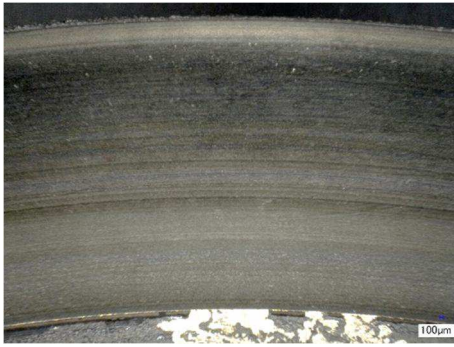
Figure 18: L6-3 valve spindle seating top view, 24,000 hours
