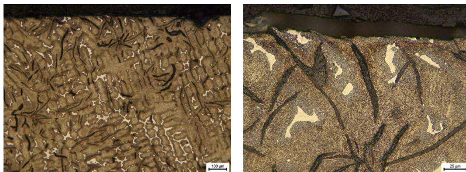
Figure 6: Cross-sectional cut of seat ring surface
