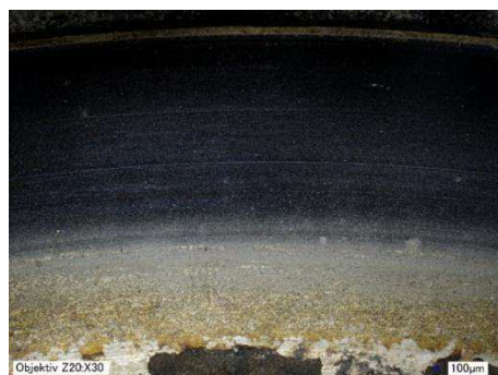
Figure 17: L2-4 valve spindle seating top view, 16,000 hours
