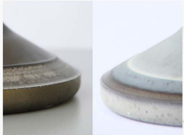
severe wear after only 2,000 hrs with a typical hardfacing alloy (left) vs. negligible wear measured in the same engine on a valve seat armored with a MW WR Superalloy after >10,000 hrs
